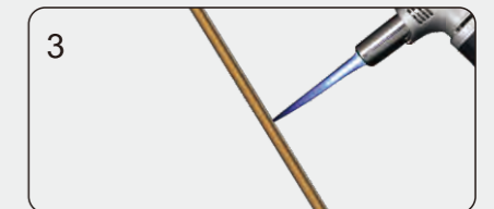
3 Prepare the tube to be expanded by heating it.
