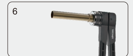
6 Press the handle down to expand the tube, allowing it to be connected with out fittings.
